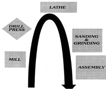
FIGURE 1-9 U-shaped Work Cell
